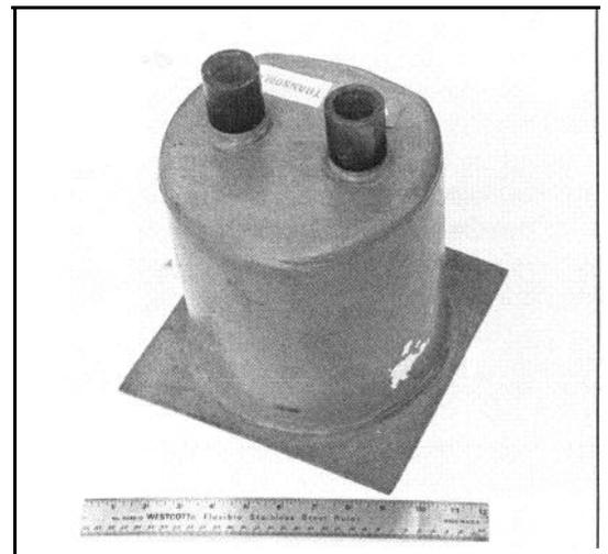
point at least three inches above the waterline at all angles of heel. The top of this stack loops downward toward the waterlift, cooling water being injected on the downhill side of the loop. The rest of the installation is identical to that of the system with the waterlift mounted below the manifold.
