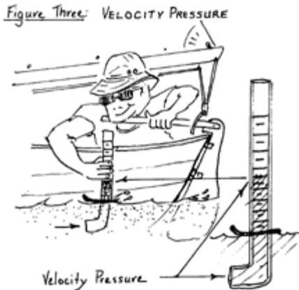
Velocity pressure is a way of expressing the speed of a fluid in terms of the pressure it causes when it strikes something. This phenomenon is used to make simple speed-measuring devices that measure the height of a column of water caused by the velocity of the water flowing past it. (See Figure Three.) Note, six knots is equal to a velocity pressure of about 19 inches, and in Figure Three the pressure is measured directly in inches of water column.
